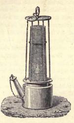
whose meshes are not too wide, over the flame of a Bunsen lamp, the flame is arrested by the gauze, although the un-
